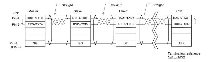
Connector diagram for 4-wire RS485 communication
